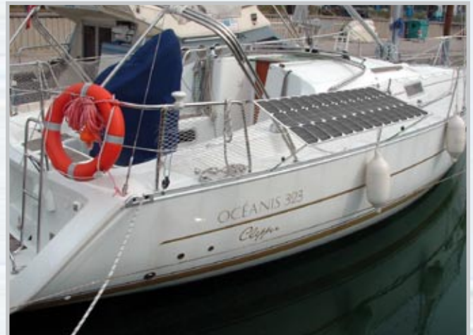
Horizontal stainless steel supporting structure
